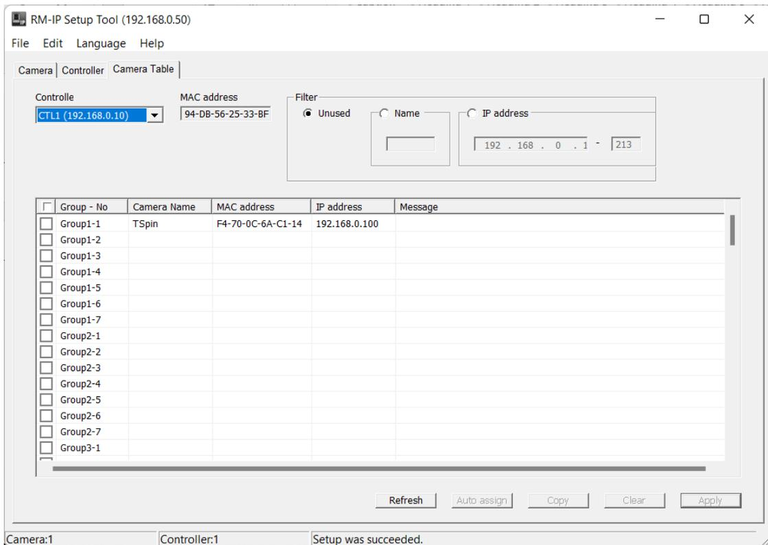
After assigning the TeleZSpin (TSpin) to the Camera Table, ensure the TeleZSpin is returned to the standard Sony VISCA over IP settings (UDP Server, Port = 52381) as described above prior to using the PTZ controller.
