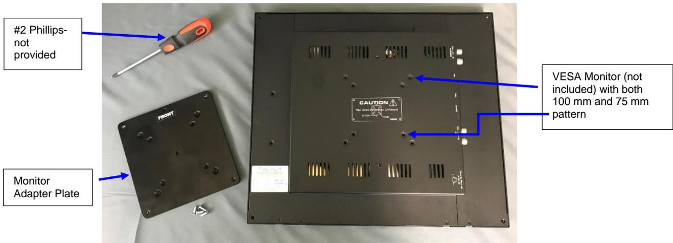
**Figure 2: Monitor adapter plate with Monitor**
