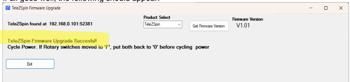
Click **Exit**, Cycle the power on the TeleZSpin. To verify, relaunch the Firmware Upgrade app and verify the firmware version
