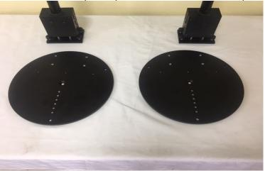
2) Remove the two Stands and place them on the baseplates. Align the Stands with the 4 thumbscrews as shown below:
