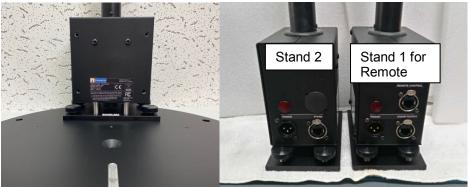
Note: The two stands are unique, Stand 1 (for Remote Control) and Stand 2. Place labels toward speakers so the Stand connections are facing each other. (Stand 1 on the left and Stand 2 on the right with speaker facing stands).
