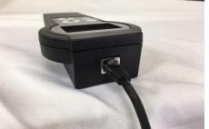
Warning! Do not plug the Ethernet cable from the Stand's Remote port into any other Ethernet devices, Routers, PC ... The +24V power could damage these devices.
