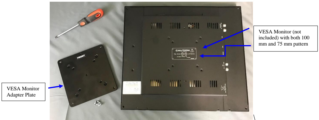
Figure 2: VESA Monitor adapter plate with Monitor
