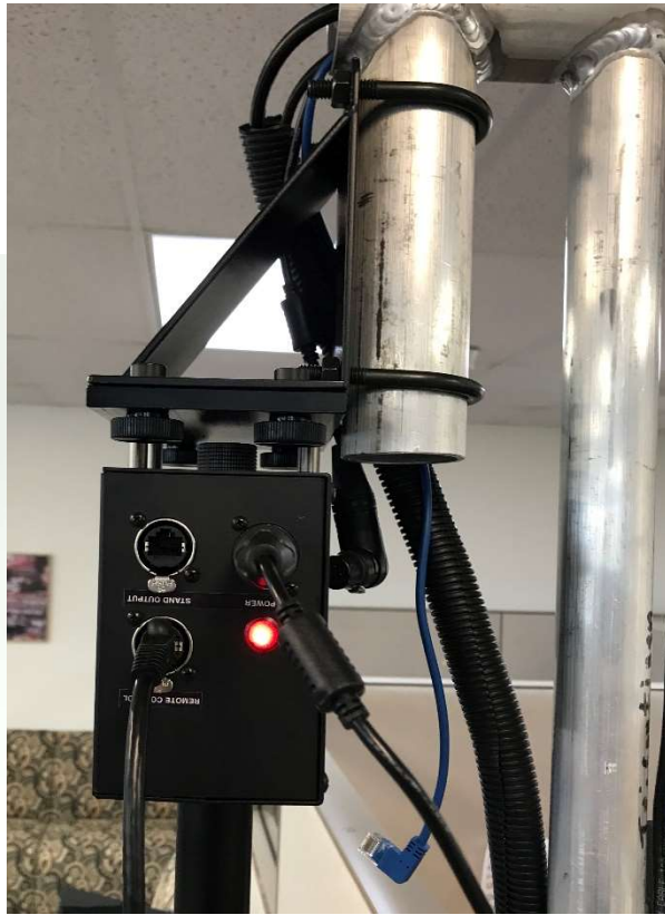
Figure 2 : PTZ Mover with Vertical Pipe-Grid Ceiling Mount Bracket (Horizontal Bracket not shown)
