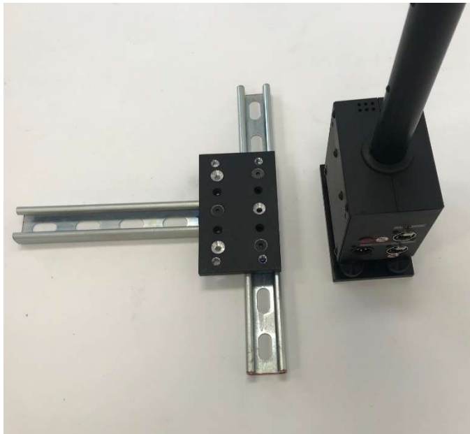
Figure 3 : PTZ Mover with Uni-Strut Ceiling Mount Bracket
